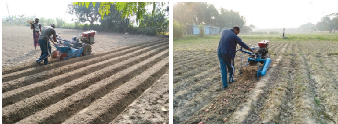
Fig. 2. Field testing of the potato planter (left) and harvester (right) machines
