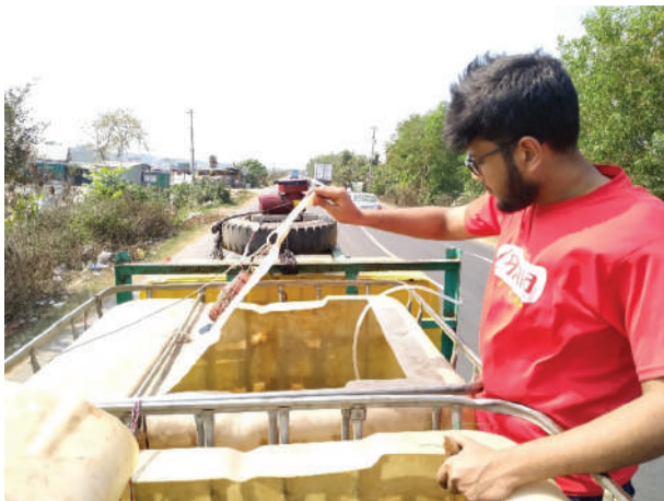
Fig. 2. Self-powered aerator-cum-water agitator used during fish transport
