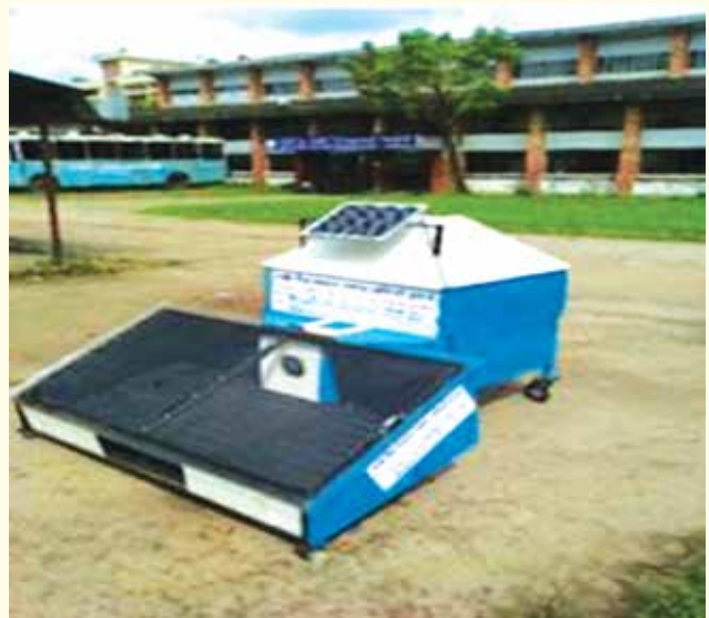
Fig. 13. Solar cabinet dryer developed by BARI for drying vegetable seeds
