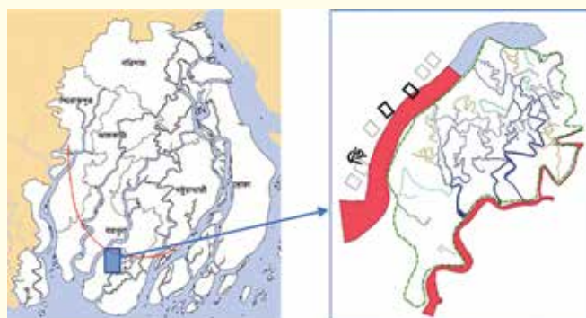
Fig. 32. Map showing river and canal system of Polder no. 44: Red and blue marks in the river indicate saline and nonsaline water, respectively
