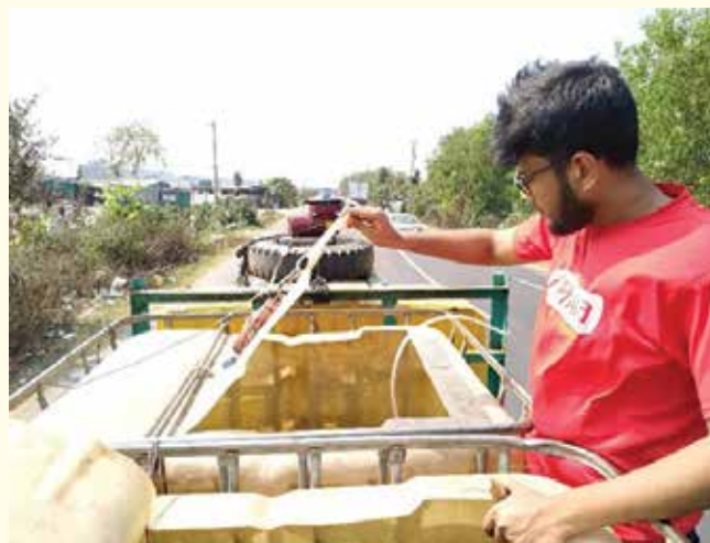
Fig. 62. Self-powered aerator-cum-water agitator used during fish transport
